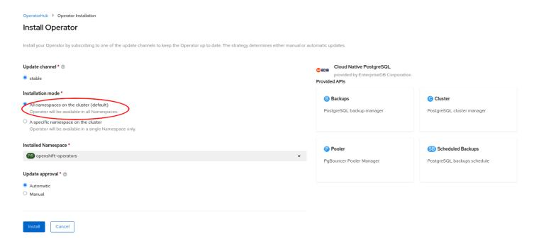
As a result, the operator will be visible in every namespaces. Otherwise, as with any other OpenShift operator, check the logs in any pods in the openShift-operators project on the Workloads > Pods page that are reporting issues to troubleshoot further.
